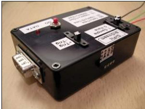
In addition, a 4 pin connector is provided, to enable connection of the optional wireless infrared transmitter modules. The optional IrTx transmitter is shown connected below.
