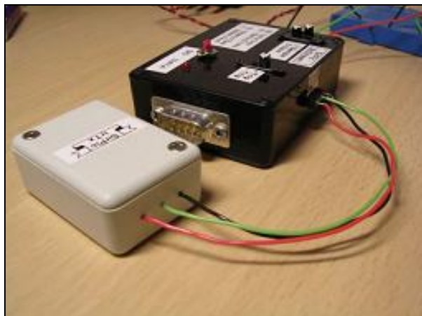
In addition, a 4 pin connector is provided, to enable connection of the optional wireless infrared transmitter modules. The optional IrTx transmitter is shown connected below.
